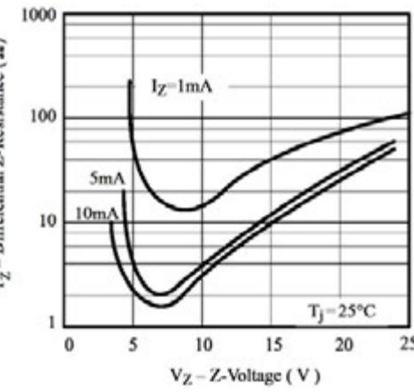
**Figure 9. Differential Z-Resistance Vz vs. Z-Voltage**
