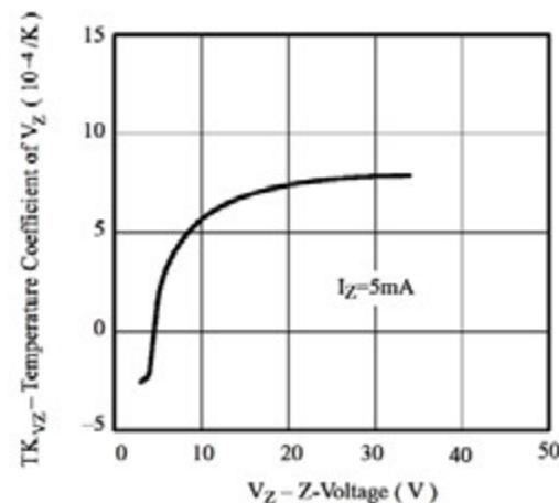
Figure 5. Temperature Coefficient of  $V_z$  vs. Z-Voltage
